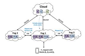
Fig.2. An example illustrating file blocks cached in multiple fogs.
