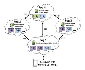
Fig.4. An example illustrating the retrieval of file blocks from neighboring fogs.
