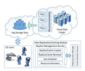
Fig.1. Proposed data replication and caching module incorporated for fog/cloud environments.
