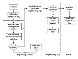
Fig.3. Flowchart illustrating the steps taken to deliver a requested file to a 5G user. If blocks are not cached in the fog serving the user, request will be sent to neighboring fogs.
